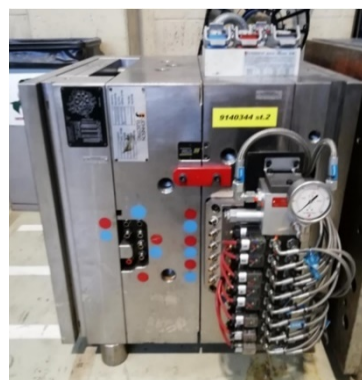
Hot runner mold installed to reduce scrap, saving 25 tons of plastic raw material per year
