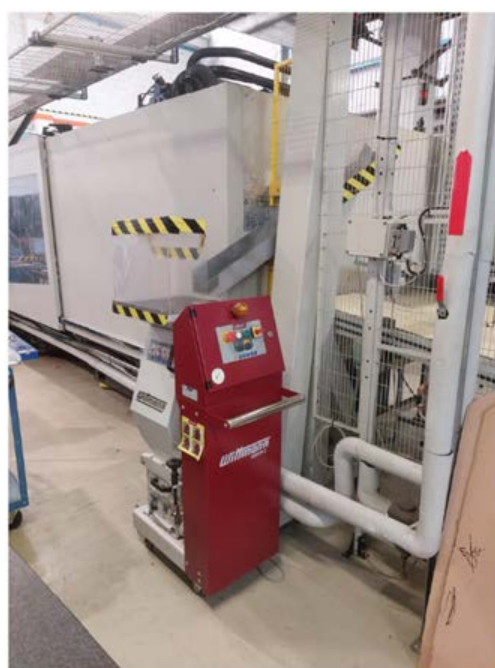
Grinding machines were added to production lines in Asti, Italy to recycle plastic sprues for reuse in production. Installed in September 2021, by the end of March 2022, these machines had already recovered 20 tonnes of material
