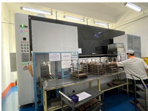
The Group purchased several hydrocarbon cleaning machines, and banned the use of ozone-depleting hydrochlorofluorocarbon solvents previously used for cleaning in its Shajing and Jiangmen, China factories
