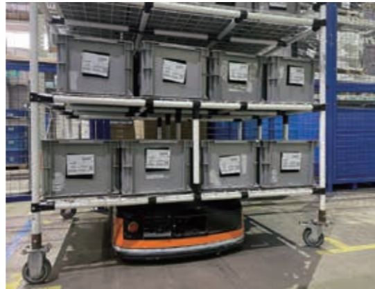
Our Wuxi, China plant has started using AGVs to eliminate manual handling risks
