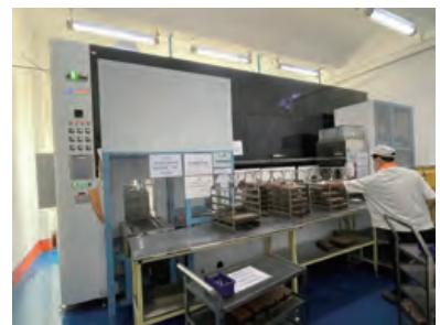
We purchased several hydrocarbon cleaning machines, and banned the use of ozone-depleting hydrochlorofluorocarbon solvents previously used for cleaning in our Shajing, China factories
